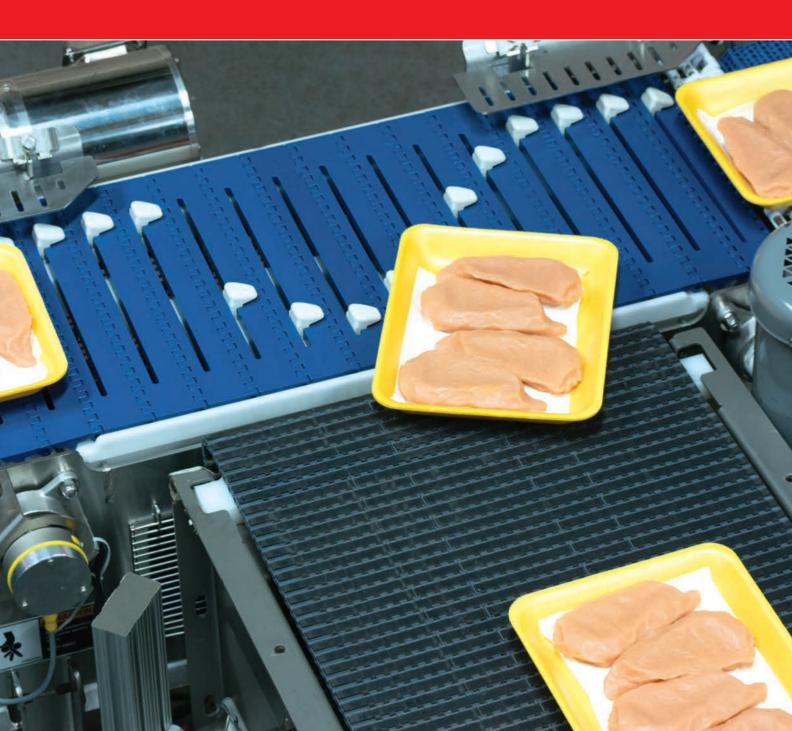
The AIM Sorter Series 800 maintains tray integrity and product direction at line speeds of up to 200 fpm (60 mpm) with gaps as small as 3 in (76 mm). The small footprint optimizes process flexibility with a 90-degree transfer, line balancing, or rework lines.
