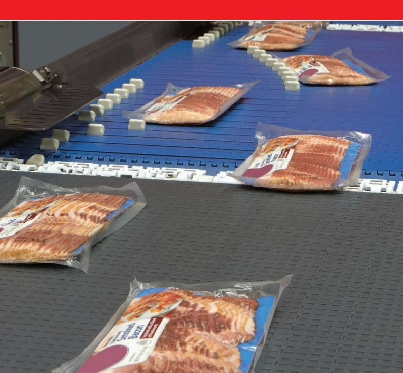
The AIM Switch Series 800 gently divides lines, while maintaining product integrity, styling, and orientation, therefore eliminating the need for non-value add labor. Process flexibility is optimized by enabling line speeds of up to 200 fpm (60 mpm) with gaps as small as 3 in (76 mm) without damaging delicate packages. Eliminating rails or other equipment from the top of the belt facilitates cleaning and prevents package jams.
